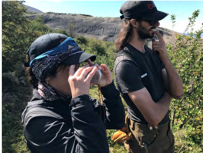
Using Clinometer to assess slope for new trail location
