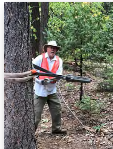
Using the grip hoist to move large dead trees – fun!
